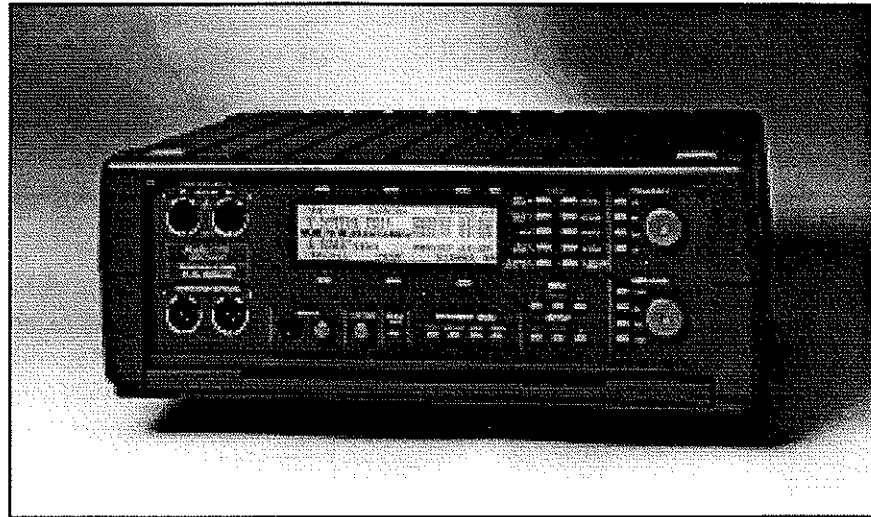
FIGURE 5-4. Portable sophisticated multi-purpose audio test system (Audio Precision Portable One). Photo courtesy of Audio Precision.
