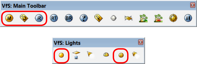
Figure 2-2: On this toolbar, we will only need the three leftmost buttons for editing materials and rendering options. The blue “R” button is the rendering button itself.
